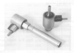
When using a diamond drilling bit with watercooling together with a normal hand drilling machine a **Dieckmann waterswivel** is necessary. Dieckmann produces waterswivels with a ø 12 mm cylindrical pin or a 1/2"-20 UNF box thread to fit the machine and a R 1/2" box thread to fit the bit.
