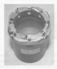
Dieckmann stratacut bits are designed for maximum core recovery and penetration rates in soft to medium formations. They are particularly applicable in soft, sticky formations where performance of large stones diamond bits may be marginal. Dieckmann stratacut non coring bits have best results in underground drilling. Stratacut tools can economically replace tungsten carbide tools.
