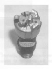
The stratacut cutters have a thin layer of polycrystalline synthetic diamonds bonded on a tungsten carbide backing. They are imbedded in a tungsten carbide matrix.
